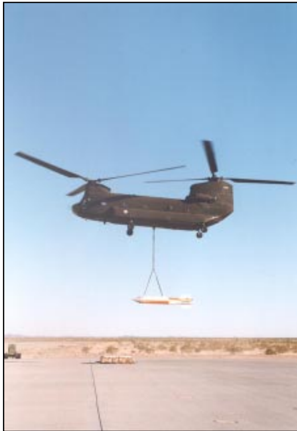
Armed Chinook? No, a Chinook from the Delta Schooners in Stockton, Calif., lifts off with a NASA X-38 Space Re-entry Vehicle test article to perform parachute tests at Yuma Proving Ground. □
