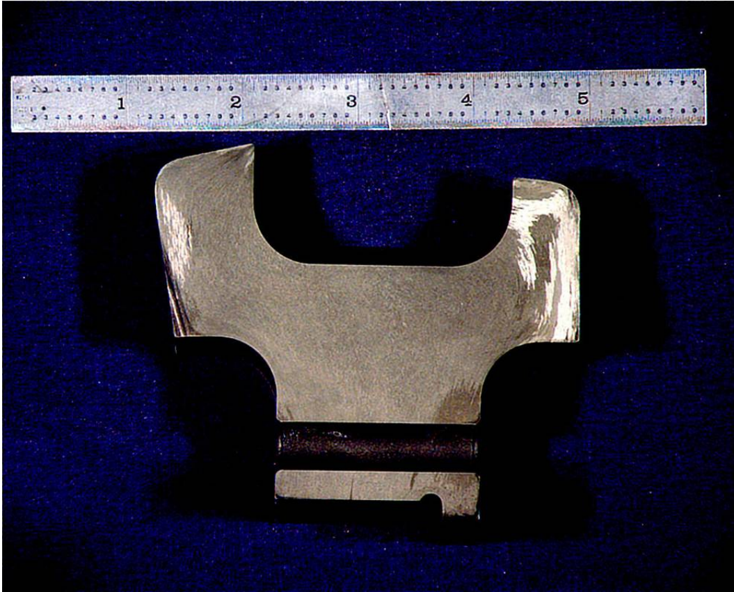
Figure 22. Macro-etch of a radial section depicting forging flow lines.
