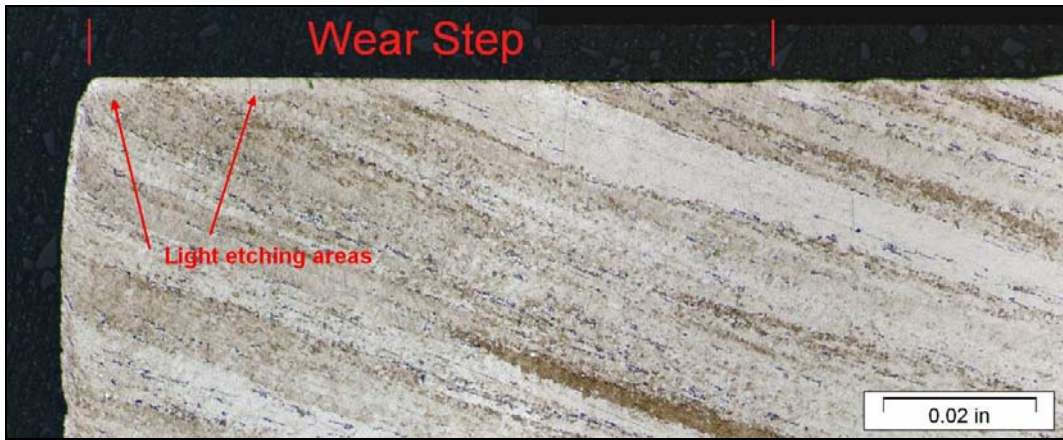
Figure 20. Microstructure near the wear step.
