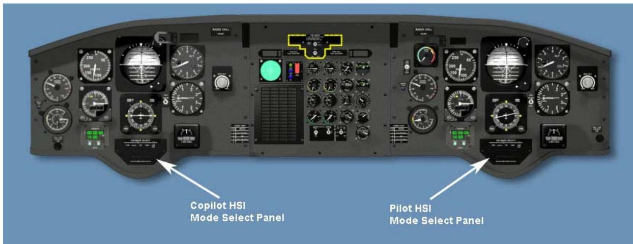
(2) The switches are push-ON type buttons and when pressed, will illuminate.
